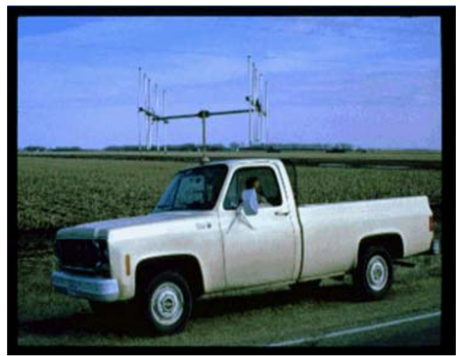
Figure 12 Truck mounted stacked Yagi antennas.
