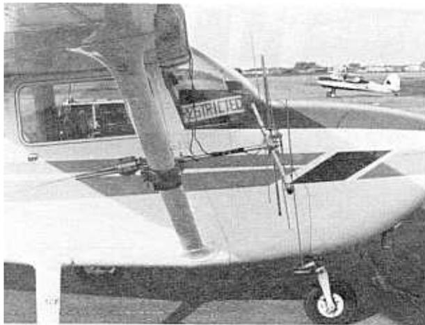
Fig. 1. Correct position of side-looking yagi antenna mounted on a Cessna 172. Front quarter view (top), side view (bottom).
