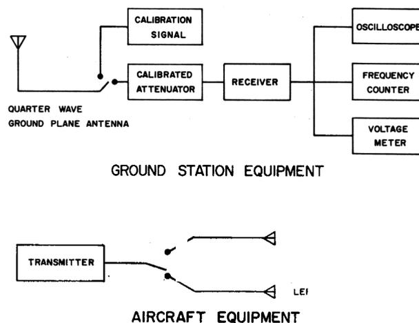
Fig. B-1. Equipment used to obtain electronic measurements during tests of antennas mounted on aircraft.
