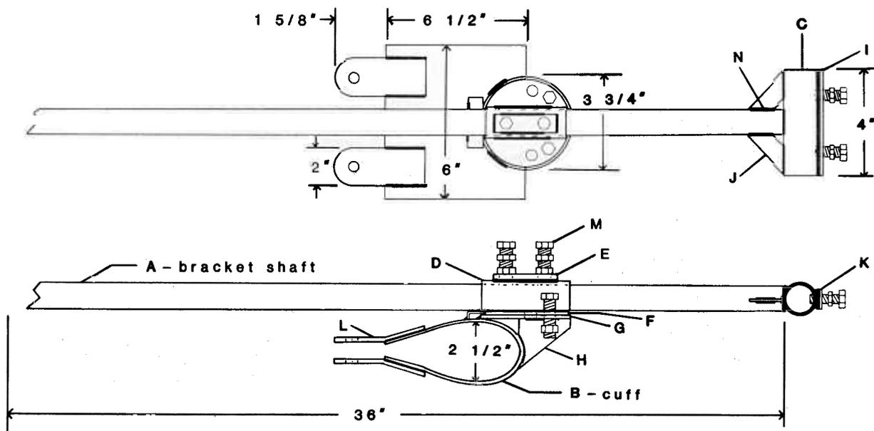
Fig. A-1. Schematic diagram of airplane wing strut yagi antenna mount. Measurements are provided in English units. Inside of cuff lined with padding to avoid scratching strut surface. All nuts and bolts should be certified for use on aircraft. These are available at any airport with repair facilities. Use lock nuts on cuff.
