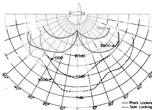
Fig. 4. Receiving antenna patterns of a loop antenna (30 MHz) mounted on a Super Cub. Readings were not obtained within the sector 20° either side of the nose and tail of the aircraft. Aircraft was flown at altitudes of about 300 and 900 m AGL.
