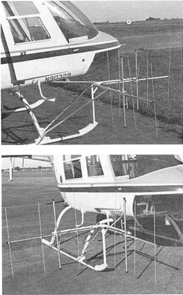
Fig. 2. Side- and forward-looking yagi antenna system designed for use on a helicopter (Bell 206B Jet Ranger). Rear quarter view (top), front quarter view (bottom).
