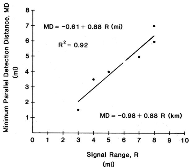
Fig. 6. Relation between minimum parallel detection range and signal range.
