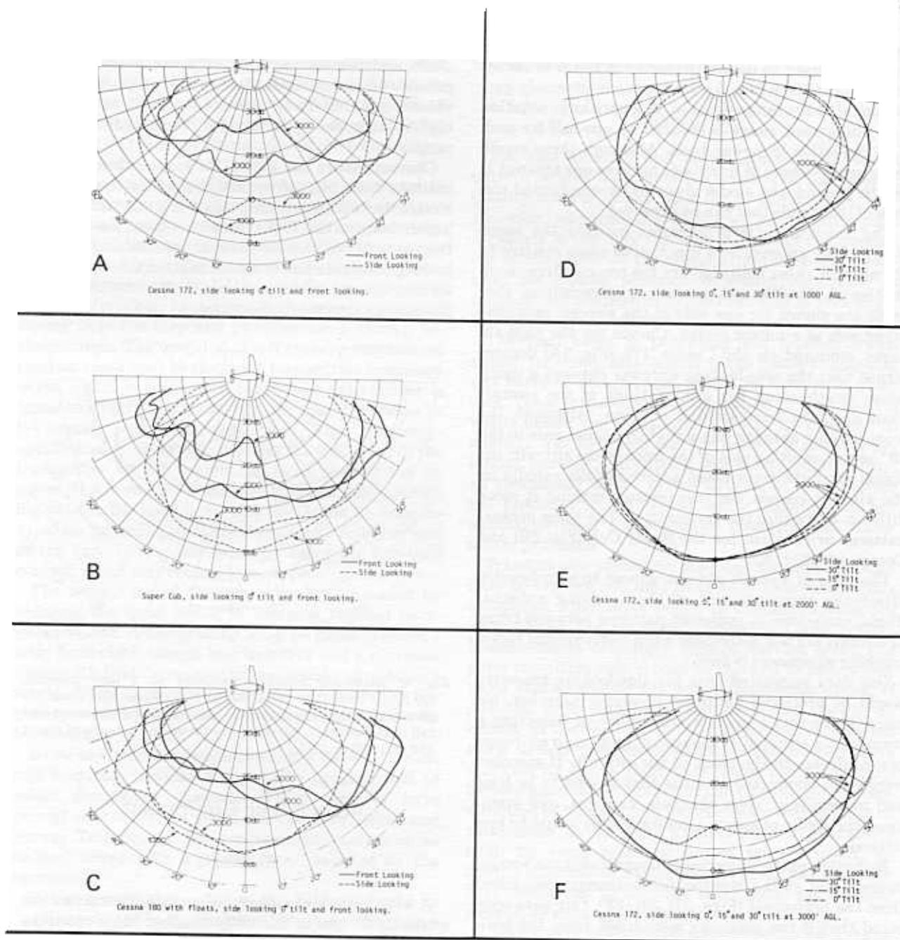
**Fig. 3.** Receiving antenna patterns of a yagi array system (164 MHz). Readings were not obtained within the sector  $20^\circ$  either side of the nose and tail of the aircraft. Aircraft were flown at altitudes of about 300, 600, and 900 m AGL.
